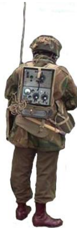
Wireless Set No18 - Paratroopers in WW-II were encouraged to land softly so as to avoid breaking all the radio valves!
