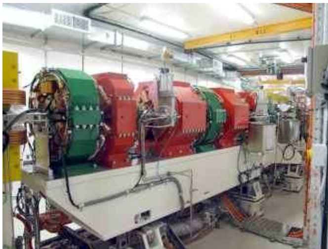
Large Electromagnets in the storage ring focus the electron beam
