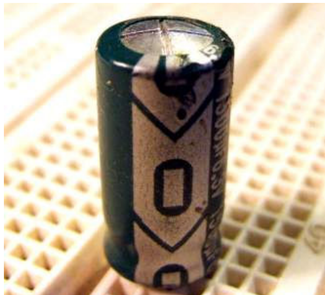
Notice the bulge in the top of this capacitor. Originally 1500uF, it now measures less than 500uF.
