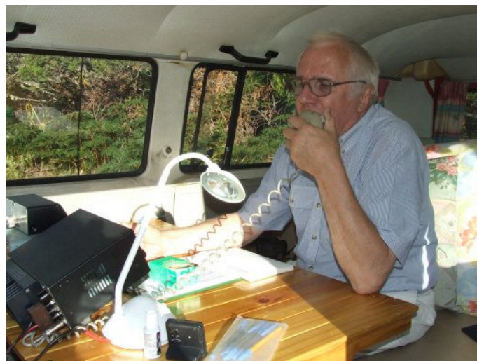
Not all field stations need to be elaborate - Gerhard VK3EWM is seen here operating from his Combi van with little more than a HF transceiver, a dipole strung between trees, and a spare car battery for power.
