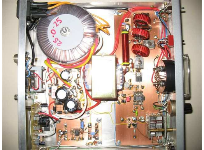
This E-Class AM transmitter is a good example of Paddy Board construction.
